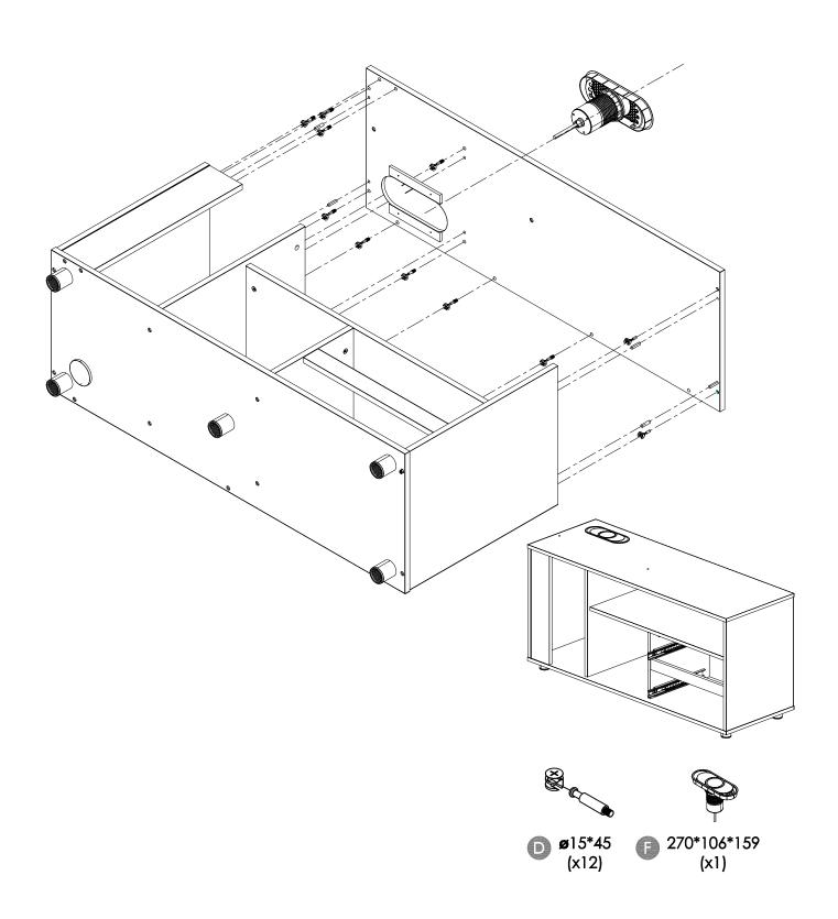
Step1. With the new 3-1 connector to fix left side drawer panle ,right side drawer panel, drawer back board, and inster the drawer bottom board into the slot
